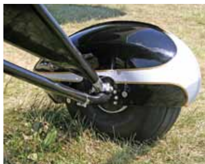
The Sportster uses easily available 800x4 tires, thanks to a special ring that sizes the original 3-inch wheel to a 4-inch wheel.
