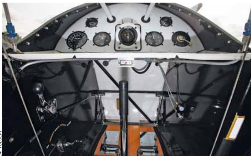
The simple and original instrument panel includes a Zenith height meter.
