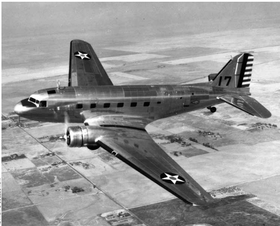
Left: As a stopgap measure, until the C-47 was available, Douglas engineers modified the DC-2. They attached a DC-2 fuselage to a DC-3 tail, added more powerful engines, and called it the C-39.
