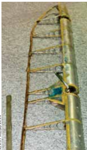
The aileron, with the fabric removed.
