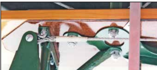
The five-tuck spliced cable was fabricated by Andrew King.
