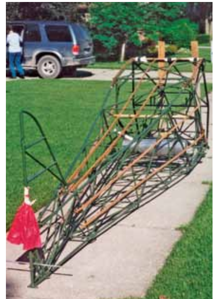
The powder-coated fuselage, with new wood stringers.
