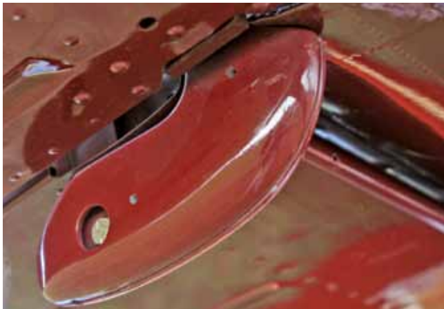
The aileron hinge fairings are made of cast aluminum.
