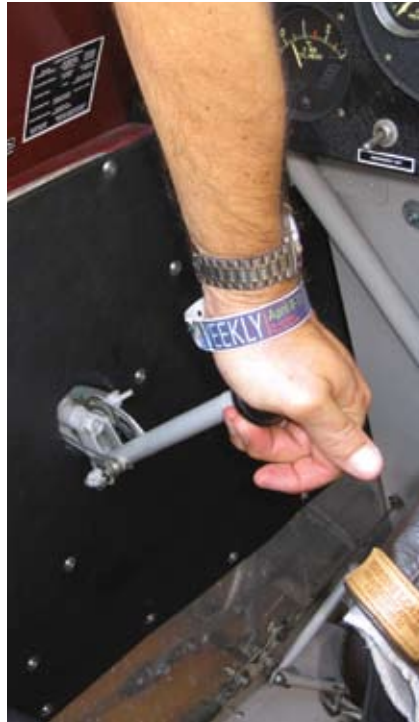
Leenhouts demonstrates the braking portion of the throttle/brake lever.
