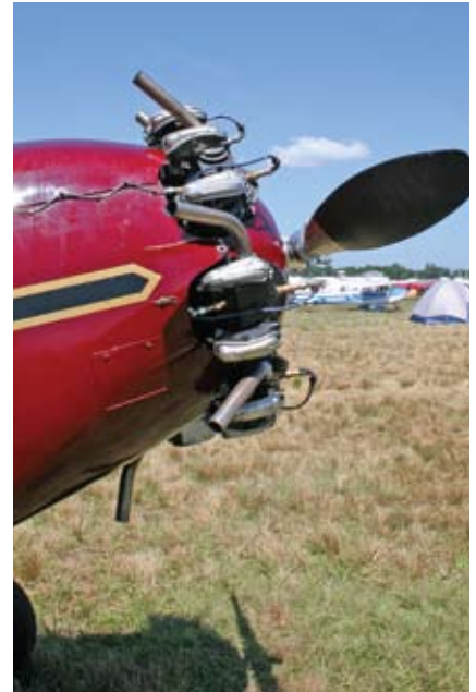
This RNF began life with a 110-hp Warner, but today it has a 145-hp Warner
